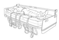
3. Make sure the chair is in its upright position. (Recline and Tilt-n-space mechanism) Align the chair so that it is correctly positioned to receive the patient and depress the central locking pedal which will automatically lock all four casters simultaneously. Place the chair into its flat position and raise the armrest, which acts as a side rail, on the non-transfer side of the chair.
