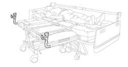
5. Attach the transfer bar to the chair brackets. Locate the silver buttons on one end of the transfer bar. Place the opposite end of the bar into the chair bracket at the foot end of the chair. Depress both silver buttons and extend the bar until the other end fits into
