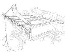
7. Pull out and extend the crank handle from the end of the transfer bar. Bend your knees and keep your back straight. Smoothly turn the crank handle so that the straps roll OVER THE TOP of the transfer bar. Keep turning until the patient is centered on the chair.
