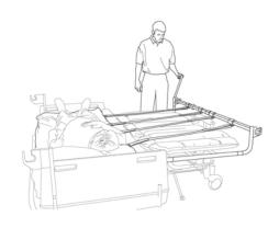
8. Remove the TranSheet. Roll the straps around the transfer bar and secure. Remove the bar from the chair brackets and store. Rotate the chair brackets back to their stored positions. Unlock the casters and slide the chair slightly away from the bed. Raise the armrest on the transfer side of the chair. Slowly raise the seatback and adjust armrests, backrest, headrest and footrest for comfort. If necessary for patient safety, secure the patient into the chair with the Barton Quick Release Belt.
